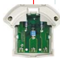
Overvoltage protection module
